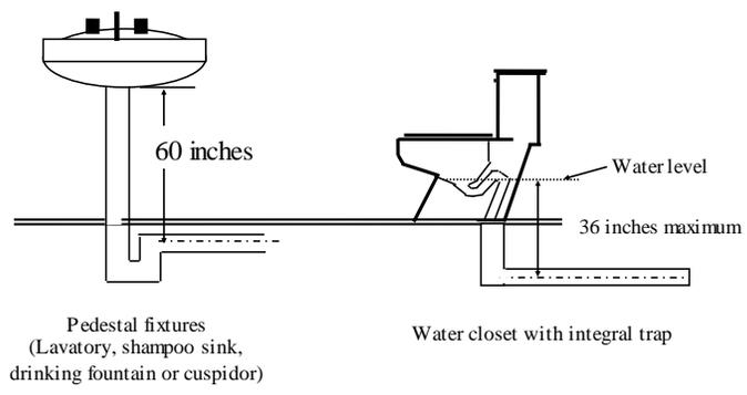
VERTICAL DISTANCE BETWEEN FIXTURE DRAIN OUTLET AND TRAP
