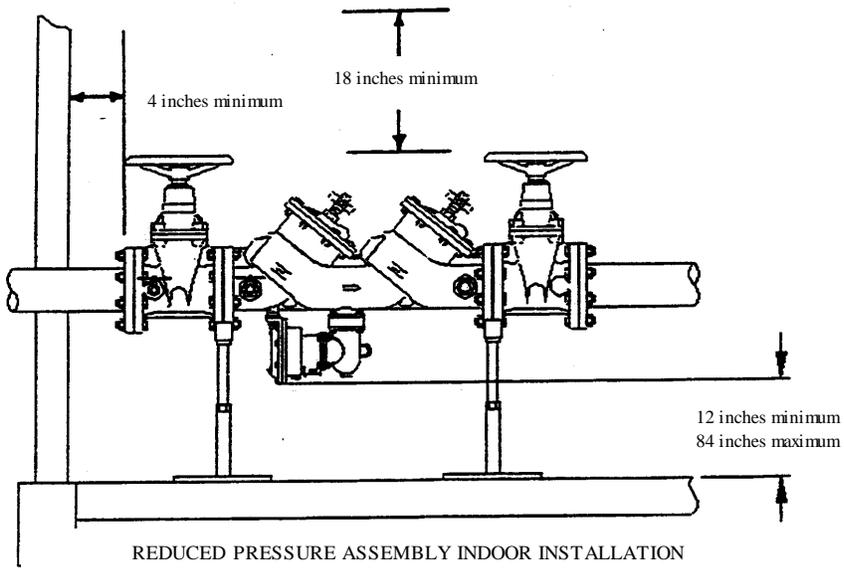
**A-82.41 (5) (f)-2. CROSS CONNECTION CONTROL ASSEMBLY INSTALLATION.**
