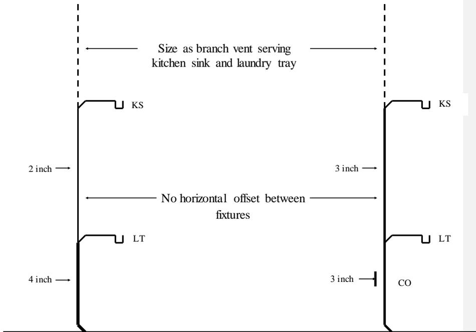
A-82.31 (17) (b) COMBINATION DRAIN AND VENT BUILDING DRAIN.
