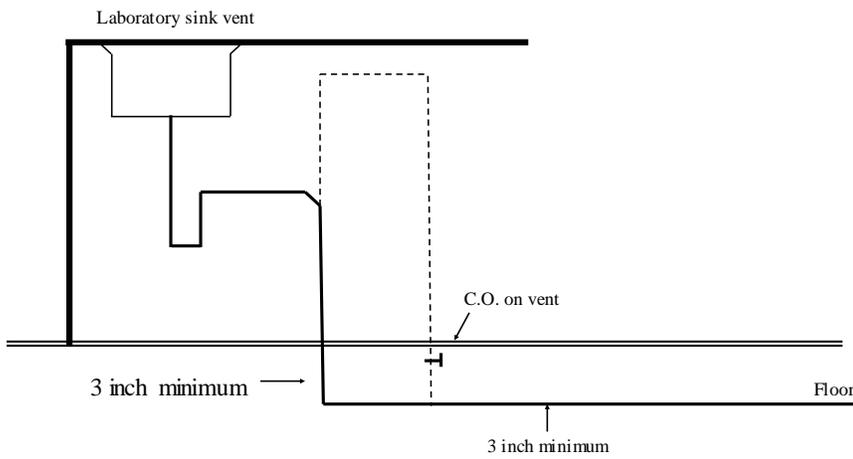
A-82.32 (4) (b) INSTALLATION OF TRAPS.
