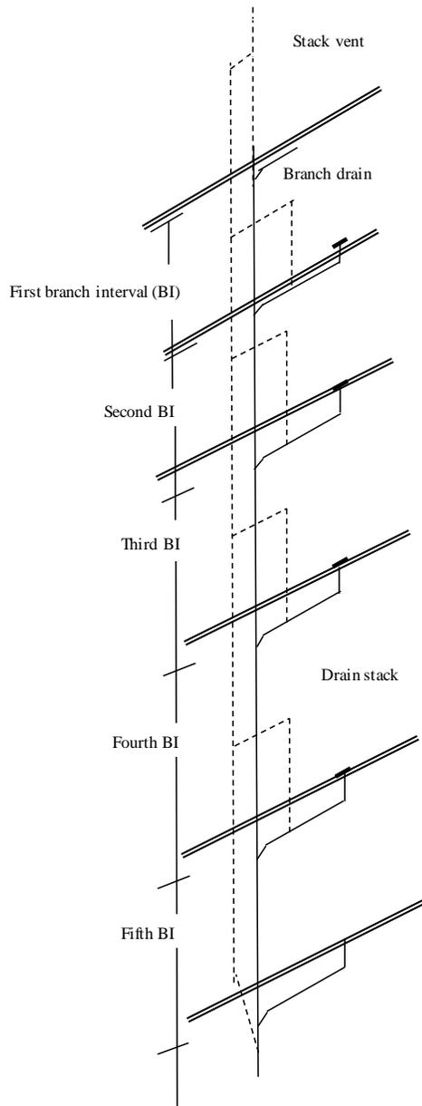
**A-82.31 (4)-2. INSTALLATION OF VENT STACK AND STACK VENT.**
