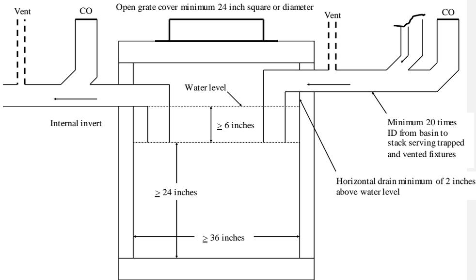
**A-82.34 (4)-6. GARAGE CATCH BASIN RECEIVING PRESSURIZED DRAINS.**
