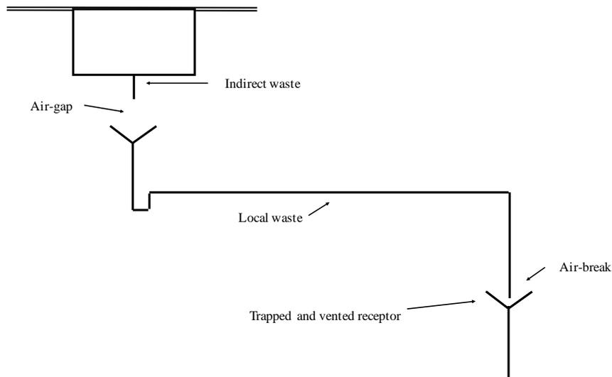
**A-82.33 (8) (a) WASTE SINKS AND STANDPIPES.**
