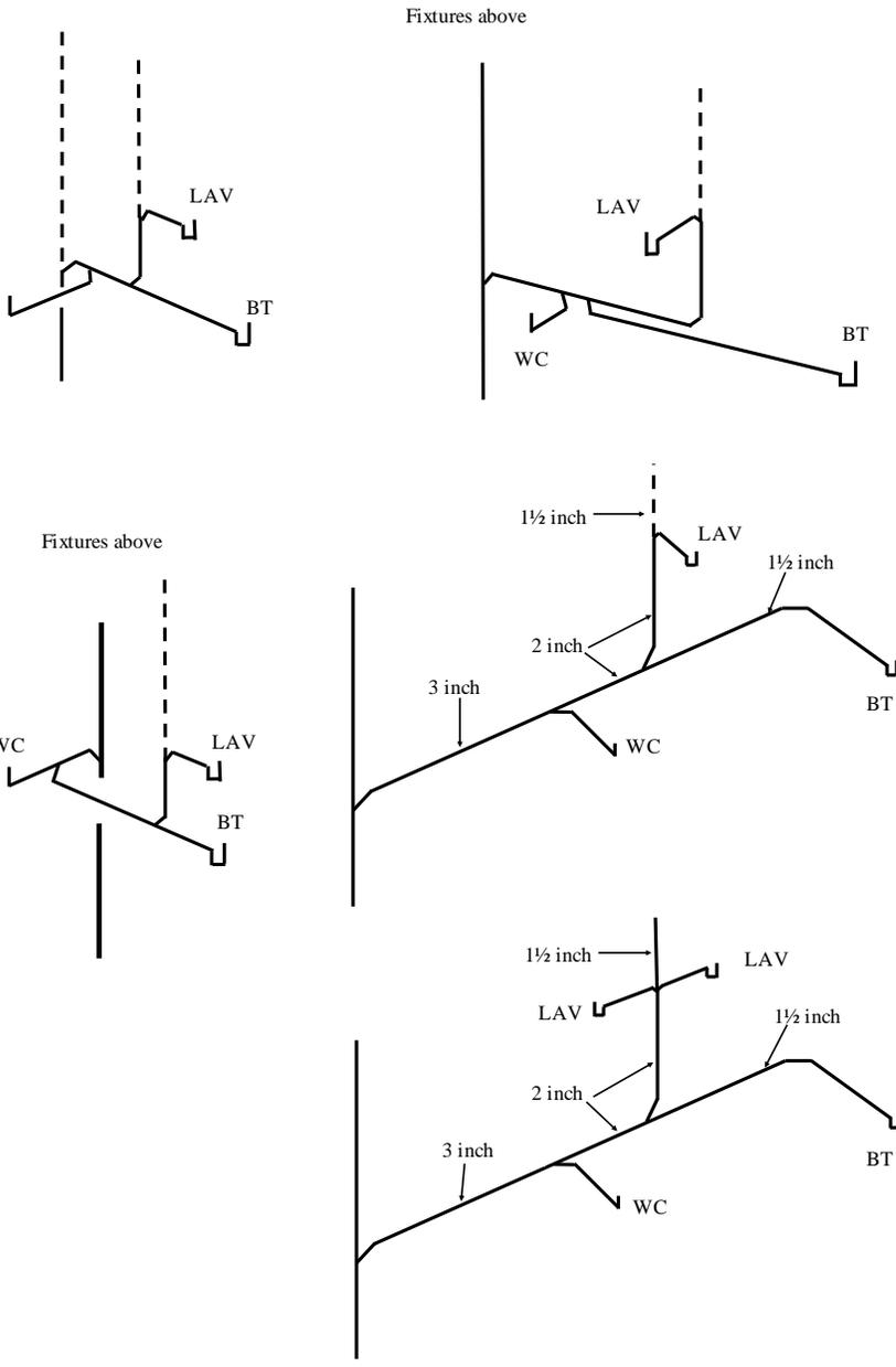
A-82.31 (13)-2. WET VENTING – FLOOR OUTLET FIXTURES.
