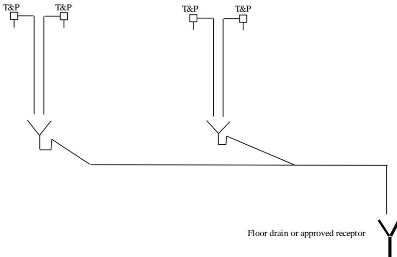
**A-82.33 (8) (d)-2. LOCAL WASTE PIPING SERVING WATER HEATER TEMPERATURE AND PRESSURE RELIEF VALVES.**
