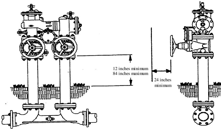
REDUCED PRESSURE ASSEMBLY OUTDOOR INSTALLATION
