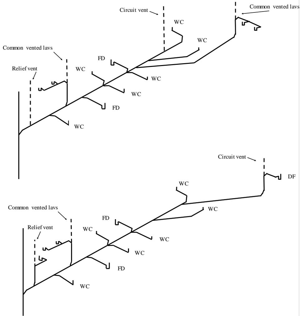
A-82.31 (11) (a) COMMON VENTS, VERTICAL, SERVING ANY TWO FIXTURES.
