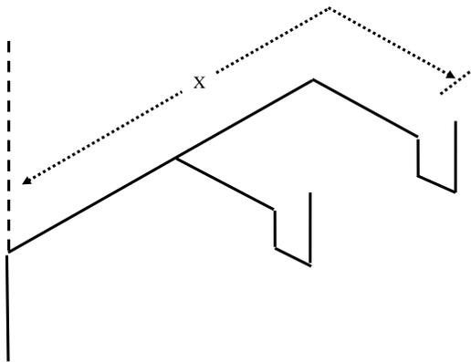
X = developed length between vent and trap
