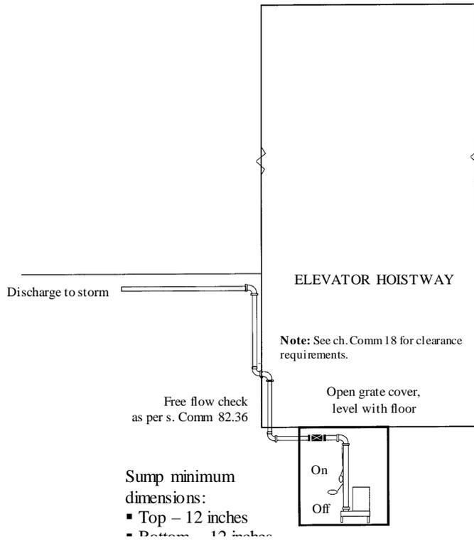
**A-82.33 (9) (f)-2. ELEVATOR PIT SUBSOIL AND FLOOR DRAINS.**
