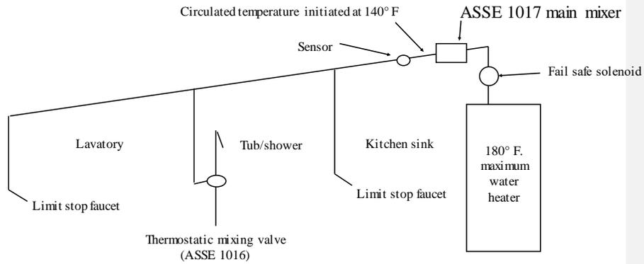
**Option 4.** Fail safe solenoid provided at main mixer meeting ASSE 1017, combination thermostatic/pressure balance mixing valve meeting ASSE 1016 and limit stop faucets at lavatory and kitchen sink.
