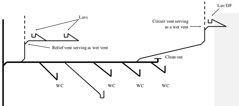
A-82.31 (14) (a) and (b) SIZING VENT STACKS AND STACK VENTS
