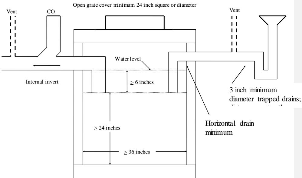
**A-82.34 (4)-3. TRAPPED FIXTURE DISCHARGING INTO GARAGE CATCH BASIN.**
