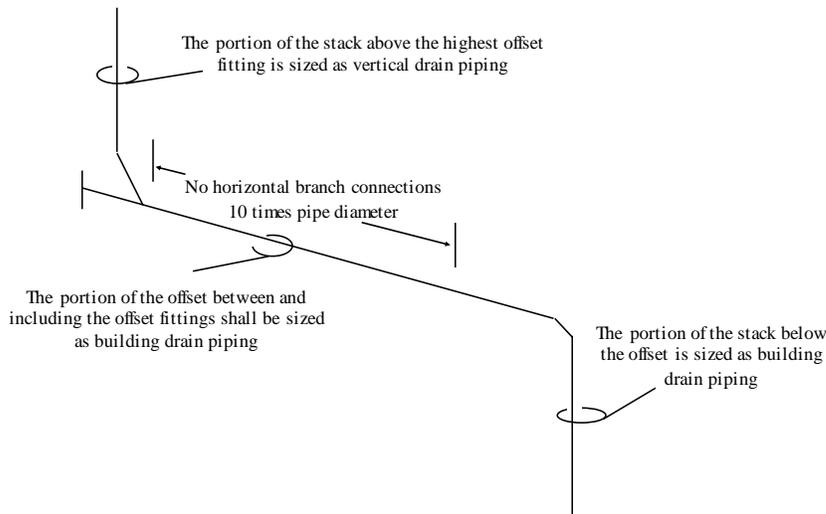
**A-82.30 (7) HORIZONTAL BRANCH DRAIN CONNECTION AT BASE OF A STACK.**
