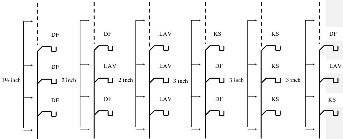
Most restrictive fixture determines stack size
