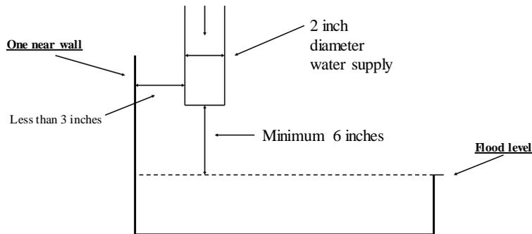
If distance is 3 times or greater than the diameter of water supply (2 inch), then the air-gap is 2 times the diameter of the water supply, (i.e. 2 x 2 = 4 inches)
