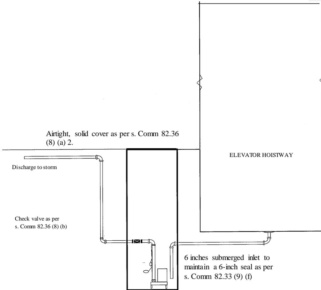
**ELEVATOR DRAIN DISCHARGE – STORM DRAIN CONNECTION**
