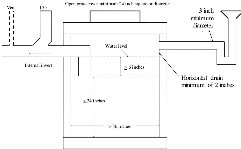
**A-82.34 (4)-4. FIXTURES WITHOUT TRAPS DISCHARGING TO CATCH BASIN.**
